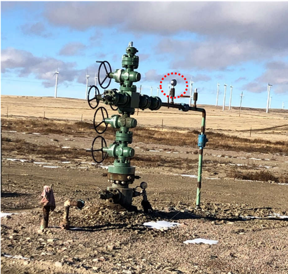
Figure A-8: A sample gas injection well, with the pressure gauge circled in red, chokes are down stream of the gauge
